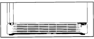
2. To level the refrigerator, use a screwdriver and turn roller adjusting screws clockwise to lower the cabinet or counterclockwise to raise the cabinet.
